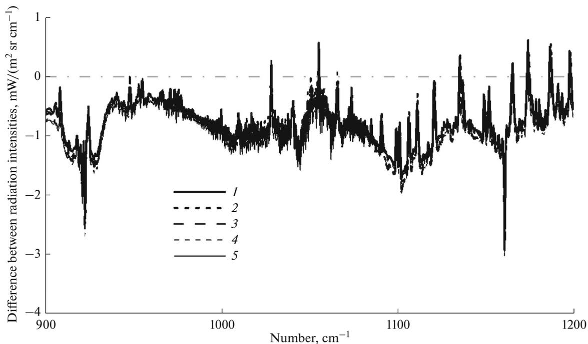
**Fig. 3.** Mean differences between measured and calculated spectra for three IR sounders and for different time periods (2015). The spectral region is the transparency window. (1) IKFS-2, February 5–6; (5) August 20–22; (2) IASI-A, February 5–6; (4) August 20–22; and (3) IASI-B, February 5–6.
