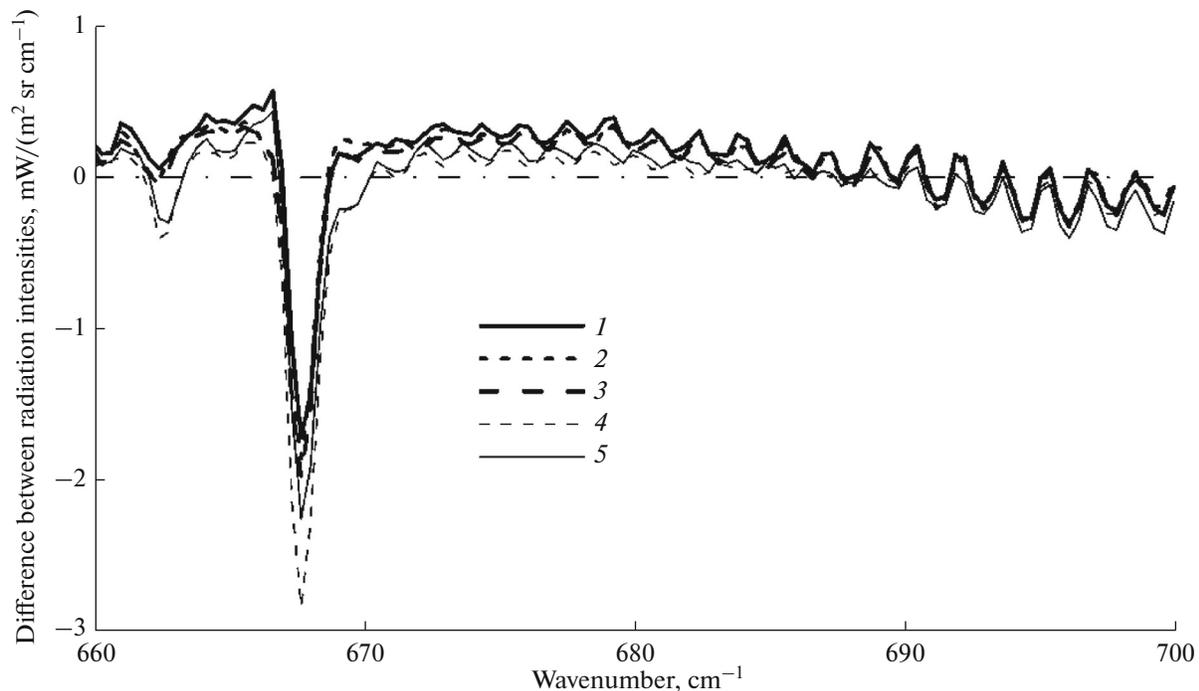
**Fig. 2.** Mean differences between measured and calculated spectra for three IR sounders and for different time periods (2015). The spectral region for the stratospheric temperature sounding. Designations of the curves: (1) IKFS-2, February 5–6; (5) August 20–22; (2) IASI-A, February 5–6; (4) August 20–22; and (3) IASI-B, February 5–6.
