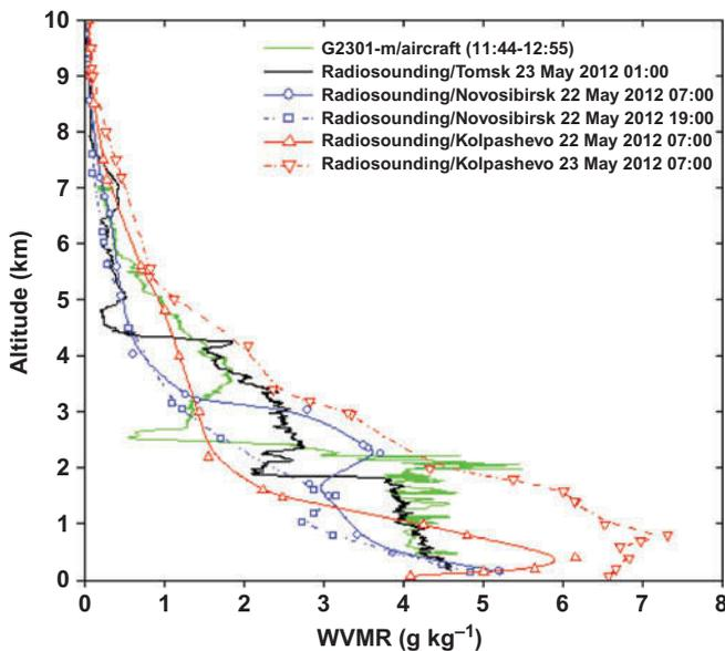
Figure 8. Vertical distribution of H<sub>2</sub>O mixing ratio (WVMR) in the troposphere obtained during aerological and aircraft sounding.
