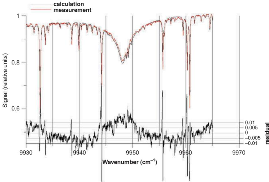
Figure 2. An example showing the presence of sinusoidal noise with the period of 17–18  $\text{cm}^{-1}$  in the residual (8:48, 22 May 2012).
