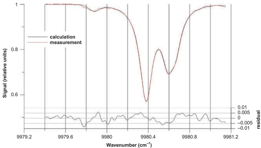
Figure 3. Measured (08:48, 22 May 2012) and calculated spectra for 9979.4–9981.5  $\text{cm}^{-1}$  spectral interval.
