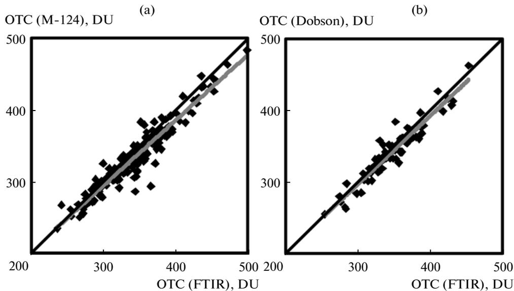
**Fig. 2.** Correlation between OTC values obtained in 2009–2012 by (a) FTIR and M-124 instruments and (b) FTIR and a Dobson spectrophotometer.
