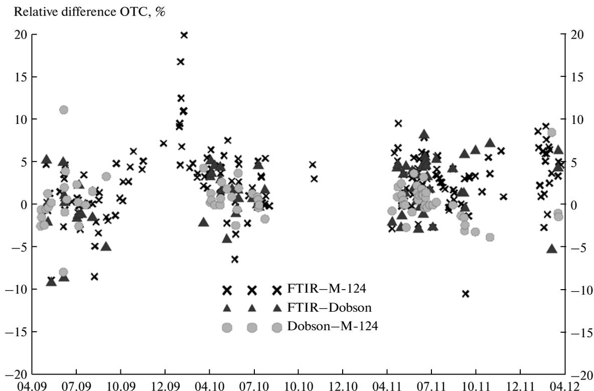
Fig. 1. Seasonal variation in errors of OTC data obtained with different ground-based instruments.
